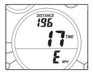
center of the large display will show the total number of hours that the elliptical crosstrainer has been used. The lower section of the large display will show an E for English miles or an M for metric kilometers. To change the unit of measurement, press the Resistance + button.
